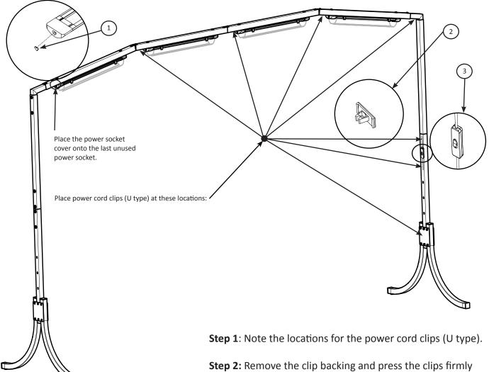
onto the frame at each location shown above.
