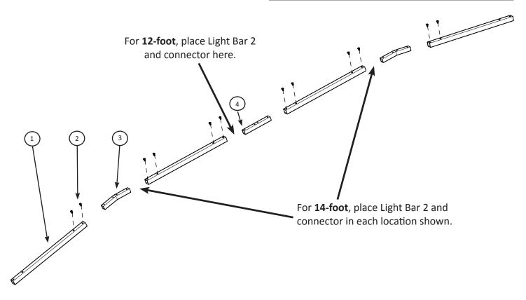
Important assembly information for 12-Foot or 14-Foot: Install the Light Bar 2 components (24 inch top tube, one straight connector and four screws) where shown in diagram above.
